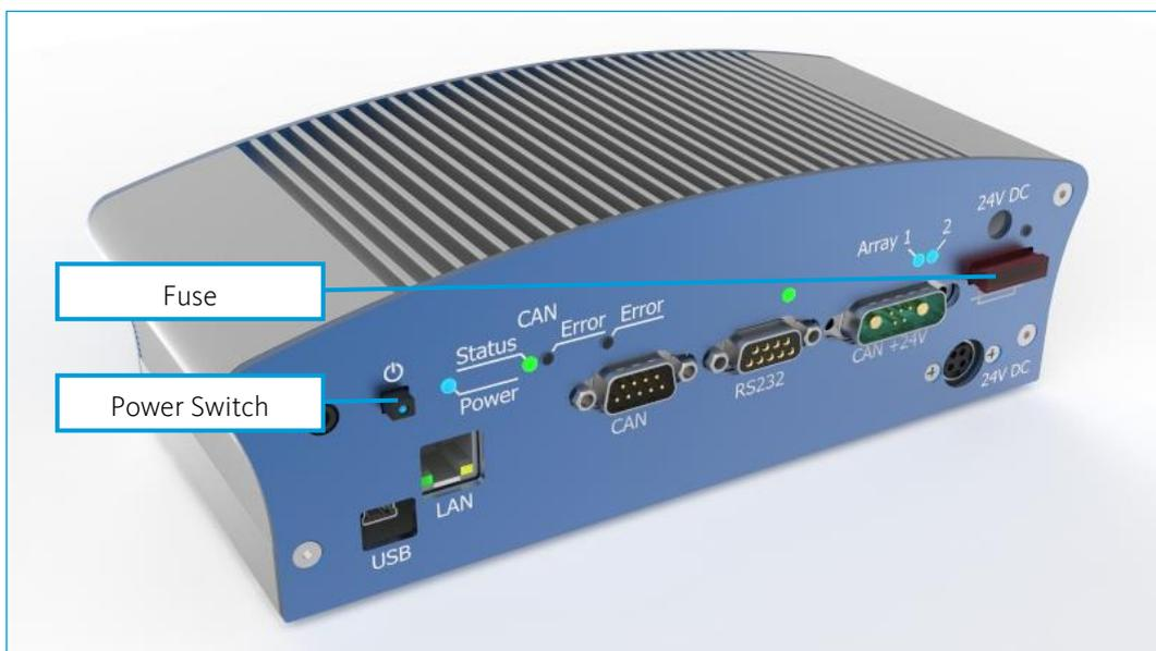
Image 1 – celled LED array controller V2
